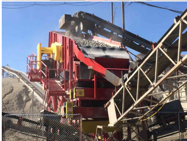
Vibratory screens can be subdivided into Inclined and Horizontal style screens.
